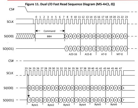
Figure 11a. Dual I/O Fast Read Sequence Diagram (M5-4= (1, 0))
