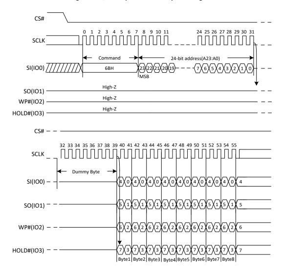
Figure 10. Quad Output Fast Read Sequence Diagram
