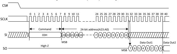
Figure 7. Read Data Bytes Sequence Diagram
