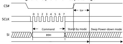
Figure 20. Deep Power-Down Sequence Diagram
