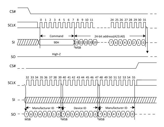
Figure 22. Read Manufacture ID/ Device ID Sequence Diagram
