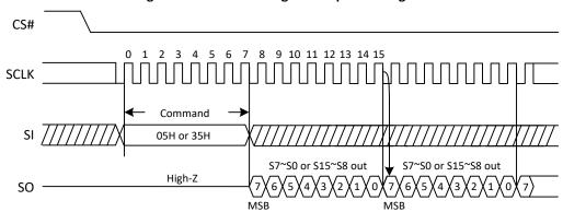
Figure 5. Read Status Register Sequence Diagram
