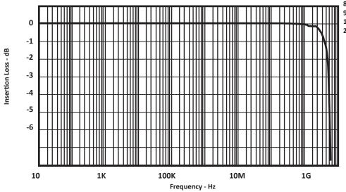
800MHz = -0.1878dB 900MHz = -0.2677db 1.8GHz = -4.1326dB 2.5GHz = -9.6452dB
