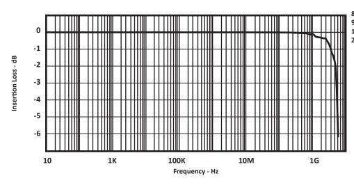
800MHz = -0.1845dB 900MHz = -0.239db 1.8GHz = -1.8755dB 2.5GHz = -3.8204dB
