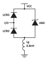
ABD - Avalanche Breakdown Diode (TVS) LCRD: Low Capacitance Rectifier Diode Lg - Lead Inductance
