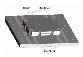
Figure 3: Component Placement
