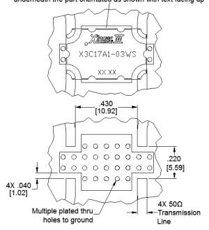
Dimensions are in Inches [Millimeters] X3C17A1-03WS Mounting Footprint
