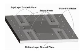
Figure 2: Solder Paste Application
