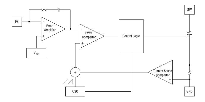
Figure 2. SDB21G Block Diagram
