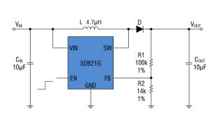
Figure 1. Basic Application Circuit
