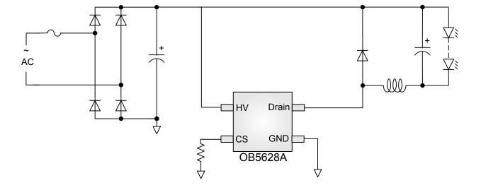
Figure 1: OB5628A Typical Application Schematic
