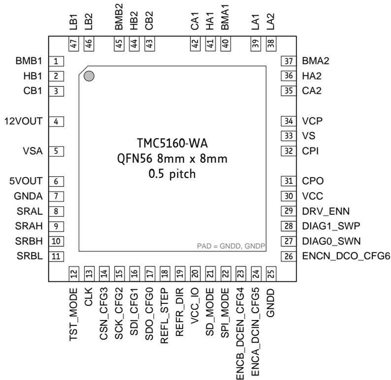
Figure 2.2 TMC5160-WA package and pinning QFN-WA (8x8mm<sup>2</sup>)
