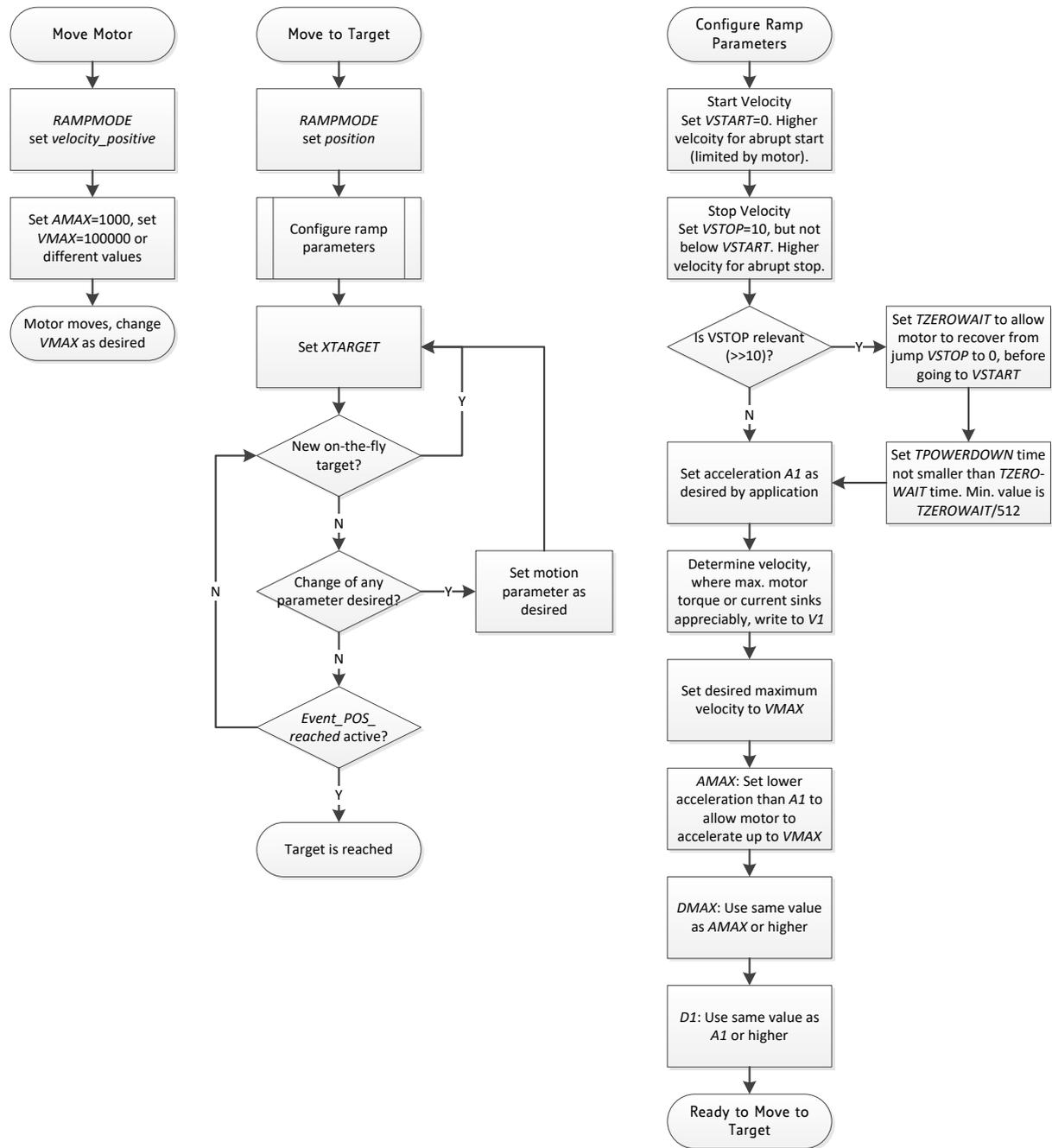
**Figure 22.3** Moving the motor using the motion controller
