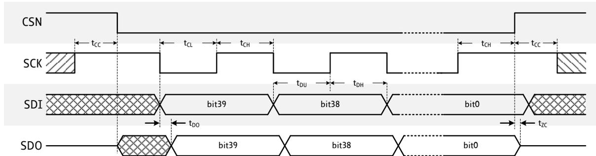
**Figure 4.1 SPI timing**
