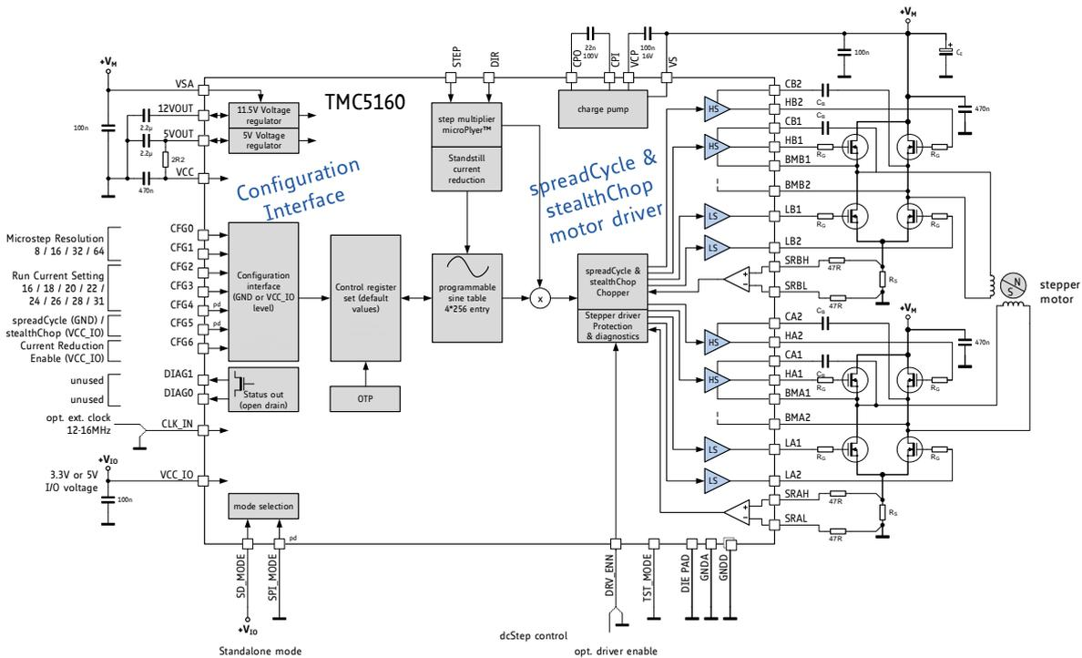
Figure 1.3 TMC5160 standalone driver application diagram
