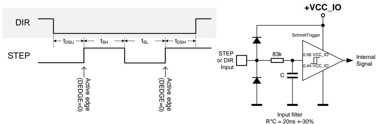
Figure 15.1 STEP and DIR timing, Input pin filter
