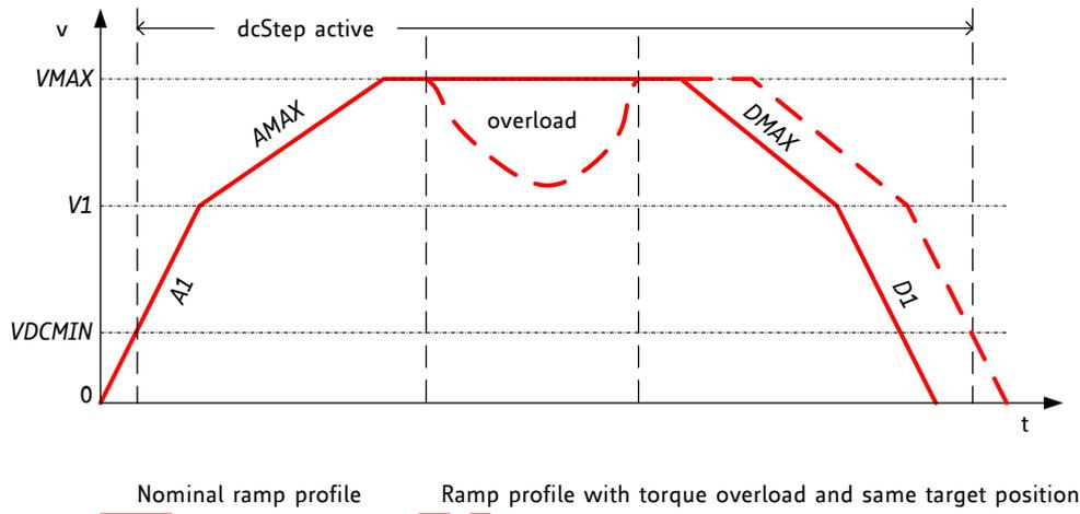
Figure 17.2 Velocity profile with impact by overload situation
