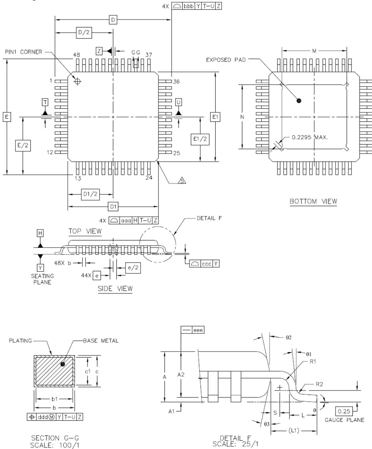
Figure 30.1 Dimensional drawings TQFP48-EP
