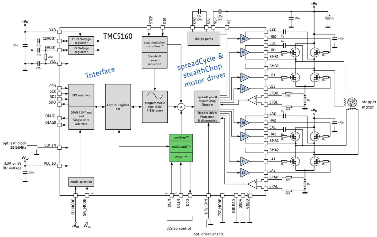
Figure 1.2 TMC5160 STEP/DIR application diagram
