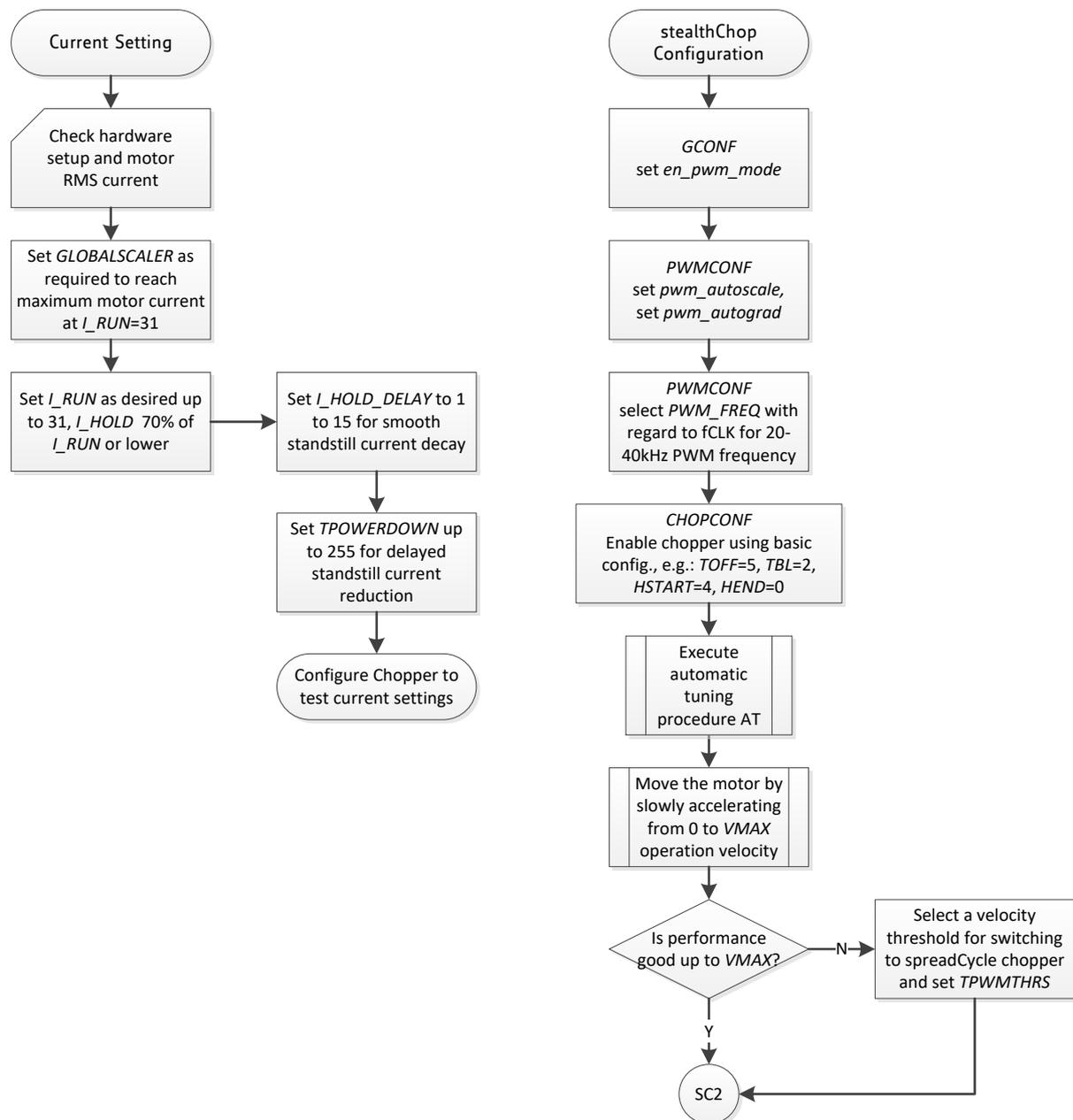
Figure 22.1 Current setting and first steps with StealthChop
