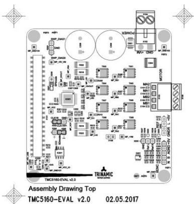
The TMC5160-EVAL is part of TRINAMICs universal evaluation board system which provides a convenient handling of the hardware as well as a user-friendly software tool for evaluation. The TMC5160 evaluation board system consists of three parts: LANDUNGSBRÜCKE (base board), ESELSBRÜCKE (connector board including several test points), and TMC5160-EVAL.
