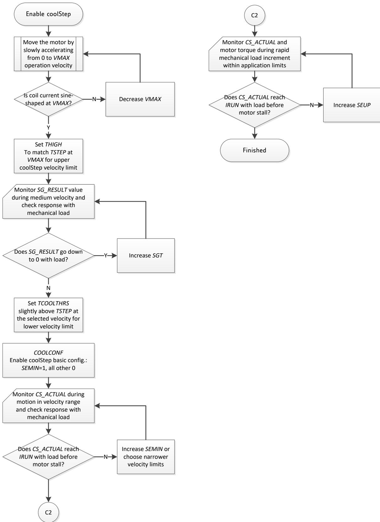
**Figure 22.4 Enabling CoolStep (only in combination with SpreadCycle)**
