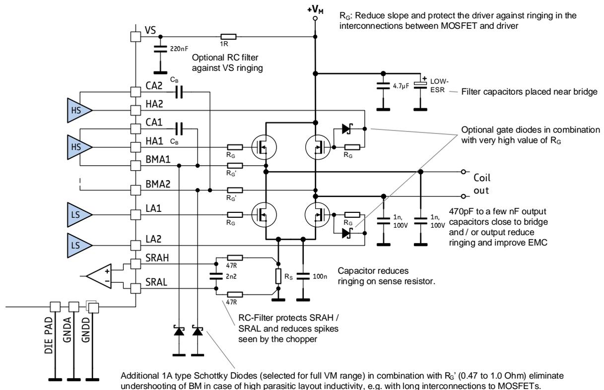
*Decide use and value of the additional components based on measurements of the actual circuit using the final layout!*
