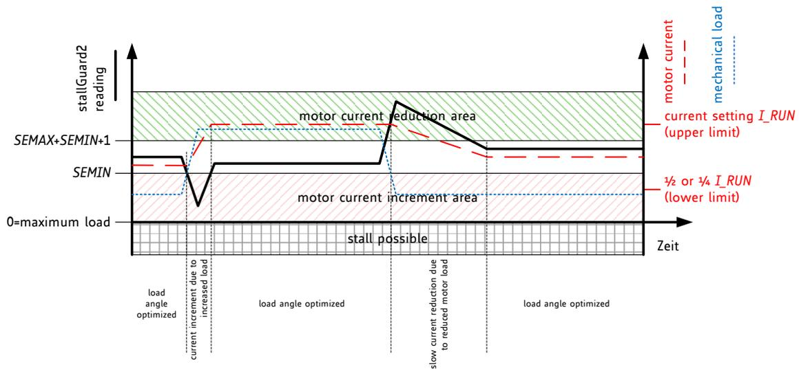
**Figure 14.1 CoolStep adapts motor current to the load**
