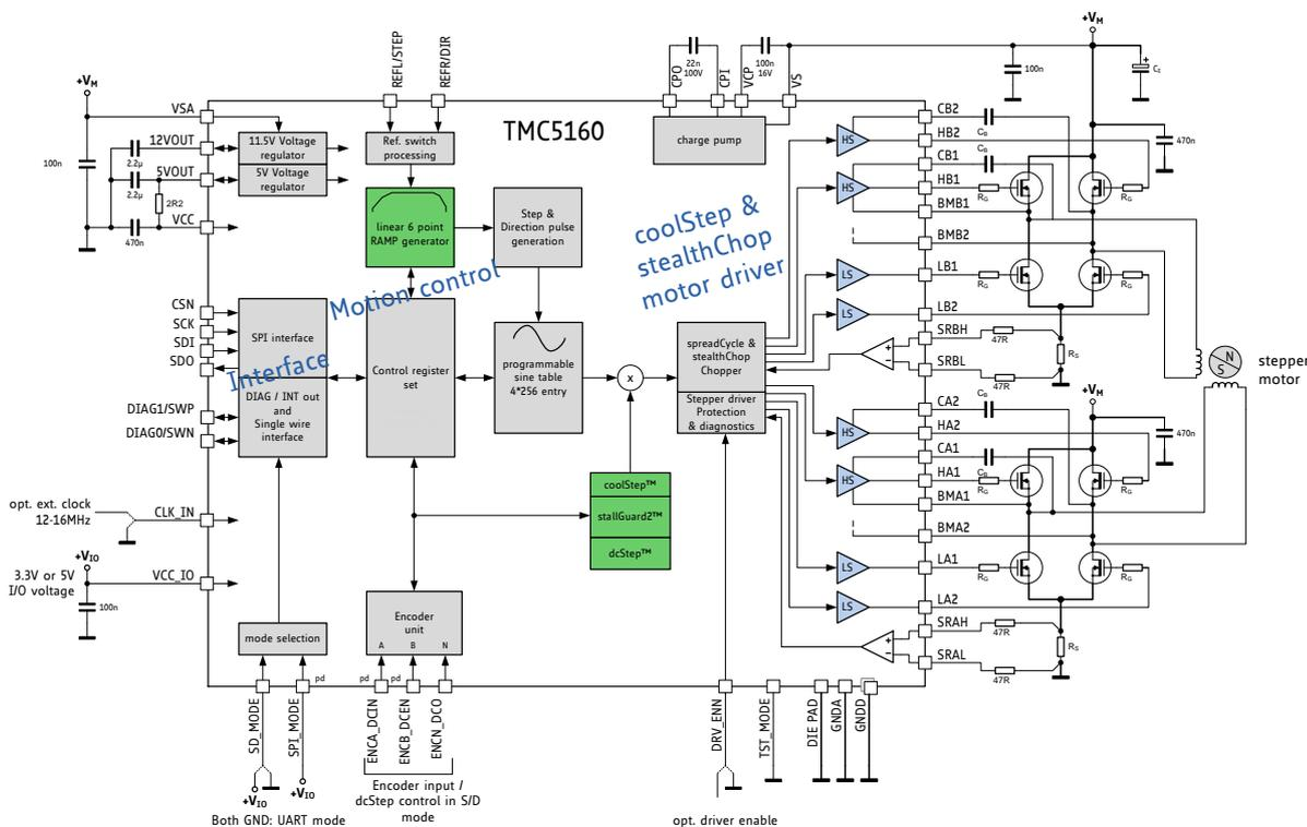
Figure 1.1 TMC5160 basic application block diagram (motion controller)
