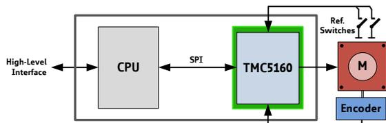
An ABN encoder interface with scaler unit and two reference switch inputs are used to ensure correct motor movement. Automatic interrupt upon deviation is available.
