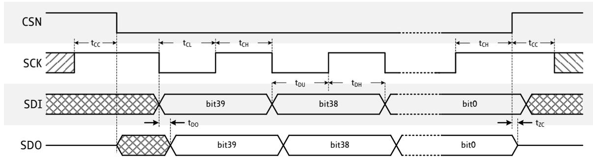
**Figure 4.1 SPI timing**
