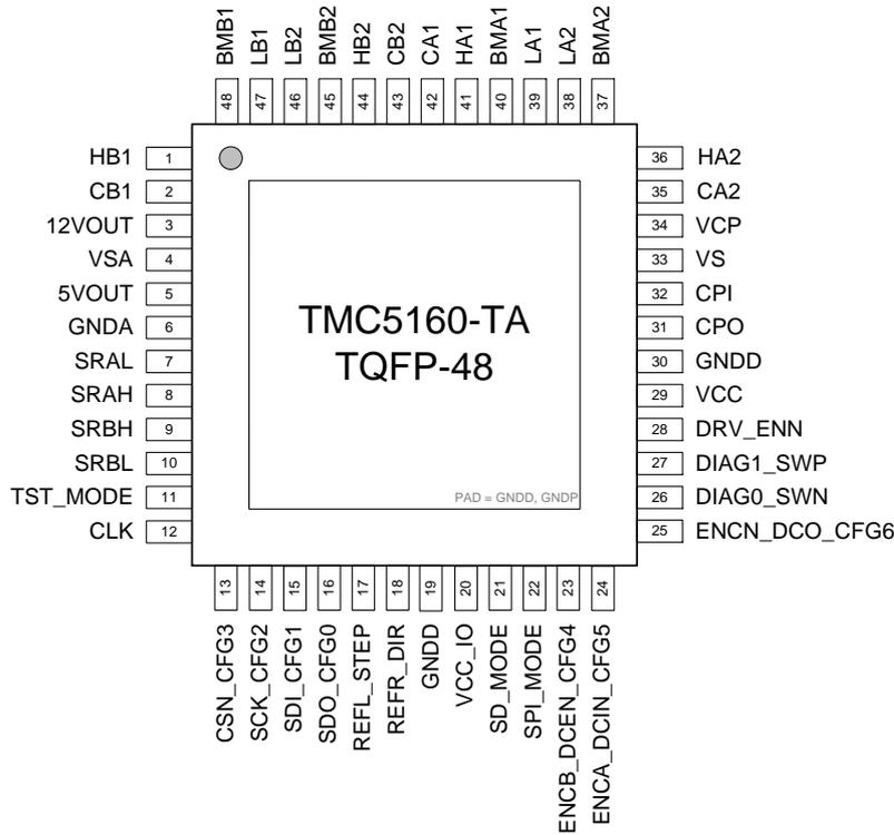
Figure 2.1 TMC5160-TA package and pinning TQFP-EP 48 (7x7mm<sup>2</sup> body, 9x9mm<sup>2</sup> with leads)
