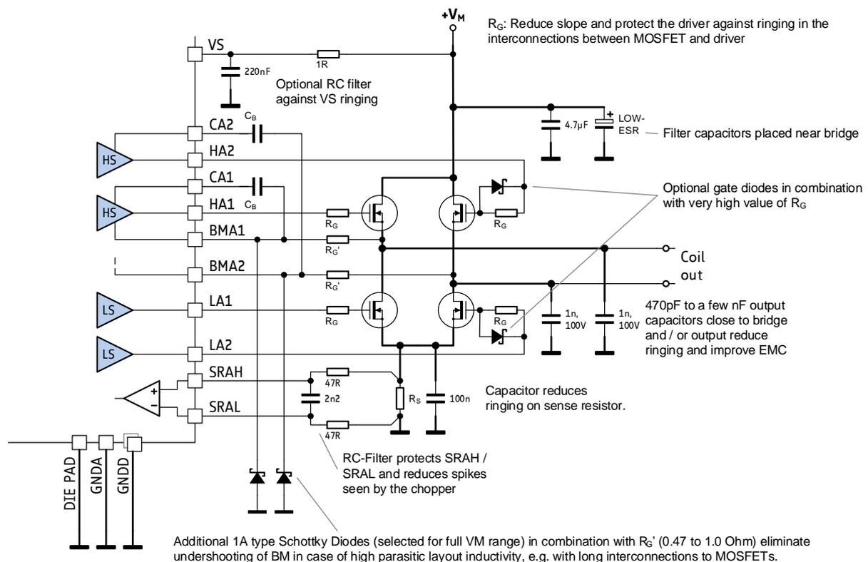
**Figure 3.5 Bridge protection options for power routing inductivity**
