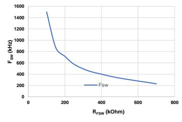
Figure 5. Switching Frequency vs FSW Resistance
