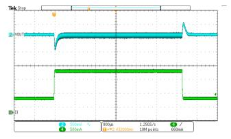
Figure 20. Load Transient (Vout=15V, lout=0.5A to 1.5A, SR=250mA/us)
