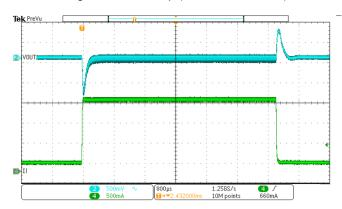
Figure 19. Load Transient (Vout=15V, lout=0.2A to 1.8A, SR=250mA/us)
