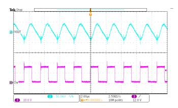
Figure 16. Switching Waveforms and Output Ripple (Vout=15V, lout=2A)
