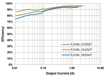
Figure 4. Efficiency, fsw=400KHz, 2-cells Battery, PFM
