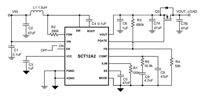
Figure 14. One Cell Battery Input, 15V Output with Load Disconnection Protection
