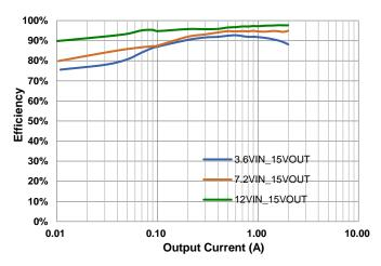
Figure 2. Efficiency, Vout=15V, fsw=400KHz, PFM
