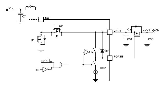
Figure 13. Load Disconnection Control
