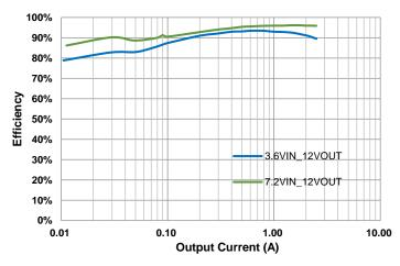
Figure 1. Efficiency, Vout=12V, fsw=400KHz, PFM
