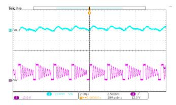
Figure 15. Switching Waveforms and Output Ripple (Vout=15V, lout=100mA)
