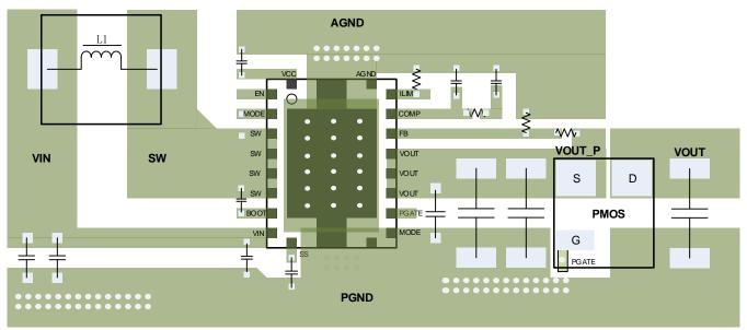
Figure 21. PCB Layout Example Top Layer
