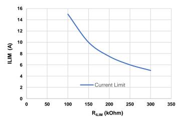
Figure 6. Inductor Peak Current Limit vs RLIM Resistance
