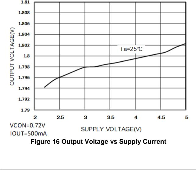
$V_{IN}=V_{RUN}=3.6V$ ;  $T_A=25^{\circ}C$ ,  $C_{IN}=10\mu F$ ,  $C_{OUT}=4.7\mu F$  and  $L=0.47\mu H$ , unless otherwise noted.
