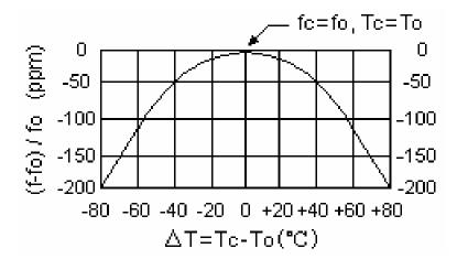
The curve shown above accounts for resonator contribution only and does not include LC component temperature contributions.
