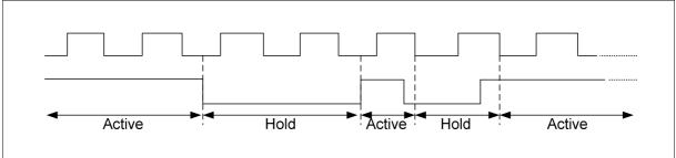
Figure 3 Hold Condition Waveform
