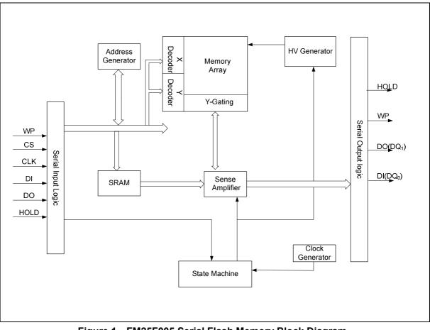
Figure 1 FM25F005 Serial Flash Memory Block Diagram
