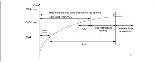
Figure 25 Power-up Timing
