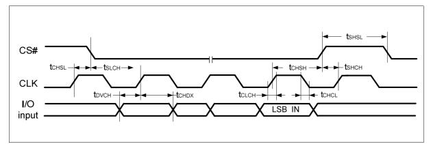
Figure 28 Serial Input Timing
