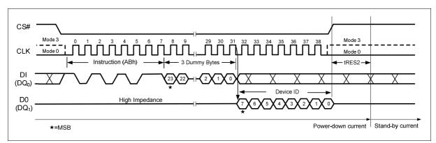
Figure 21 Release Power-down / Device ID Instruction
