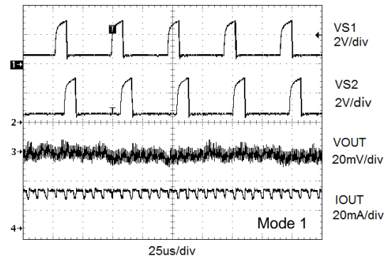
Digital PWM Dimming (1kHz, 20% duty cycle)
