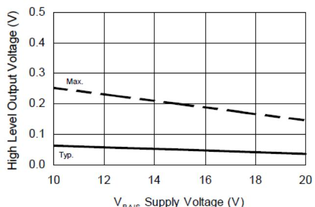
**Figure 14B. High Level Output vs. Supply Voltage**
