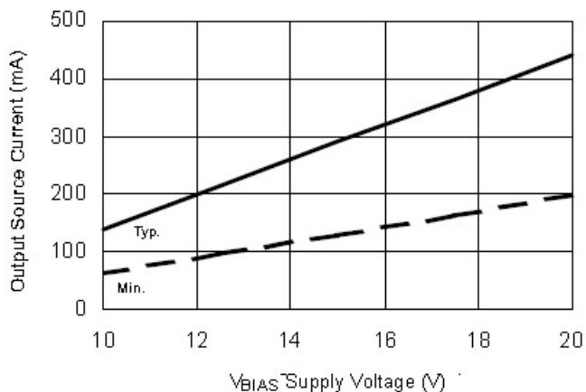
**Figure 23B. Output Source Current vs. Supply Voltage**
