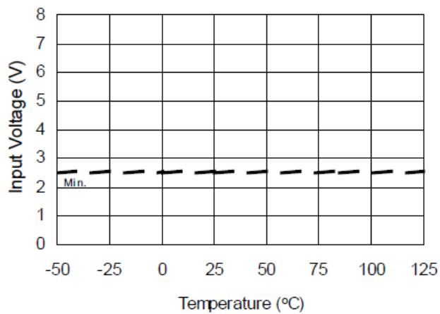
**Figure 12A. Logic "1" Input Voltage vs. Temperature**
