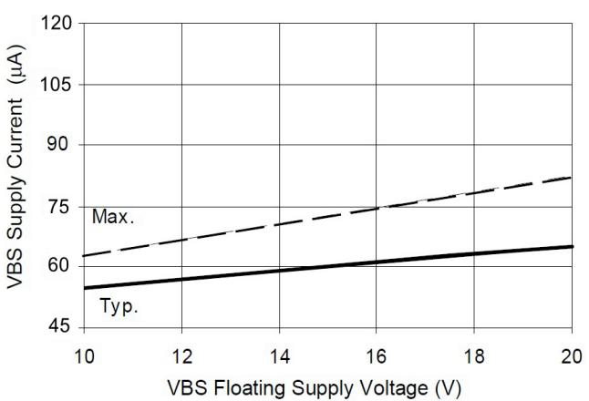
**Figure 17B. V<sub>BS</sub> Supply Current vs. Voltage**
