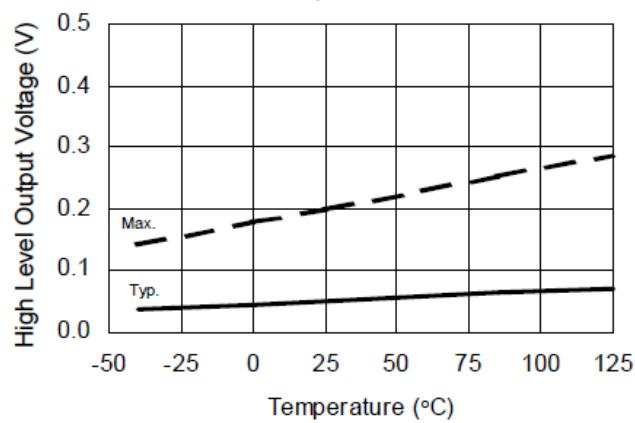
**Figure 14A. High Level Output Voltage vs. Temperature**
