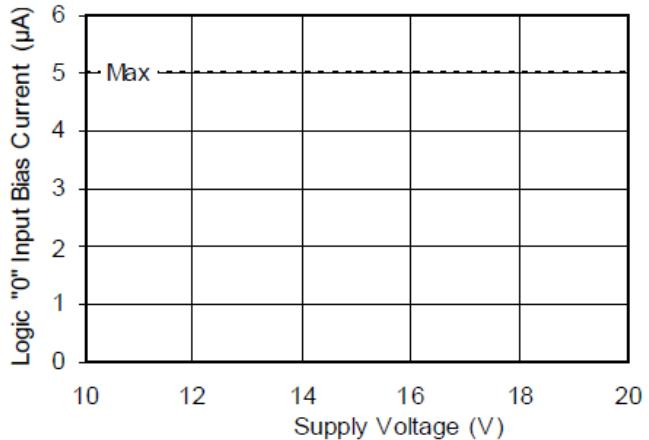
**Figure 13B. Logic "0" Input Bias Current vs. Voltage**
