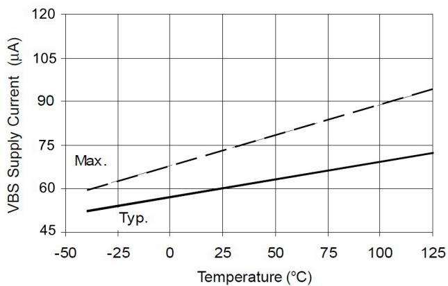
**Figure 17A. V<sub>BS</sub> Supply Current vs. Temperature**
