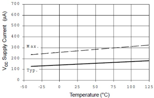
**Figure 18A. V<sub>CC</sub> Supply Current vs. Temperature**
