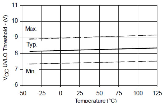
**Figure 21B. V<sub>CC</sub> Undervoltage Threshold(-) vs. Temperature**
