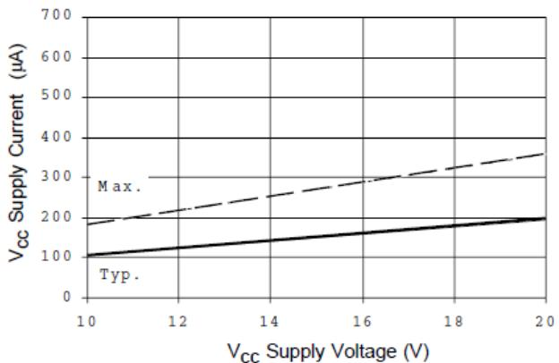
**Figure 18B. V<sub>CC</sub> Supply Current vs. Voltage**
