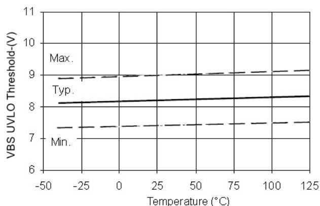
**Figure 22B. VBS Undervoltage Threshold(-) vs Temperature**
