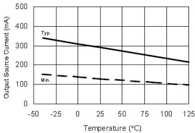
**Figure 23A. Output Source Current vs. Temperature**
