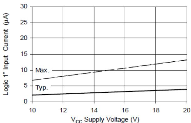
**Figure 19B. Logic "1" Input Current vs. Voltage**
