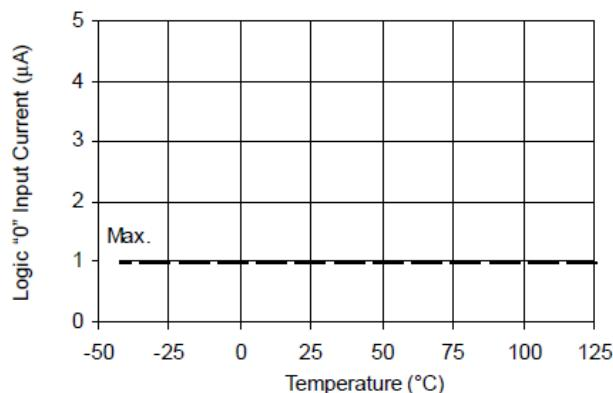
**Figure 20A. Logic "0" Input Current vs. Temperature**
