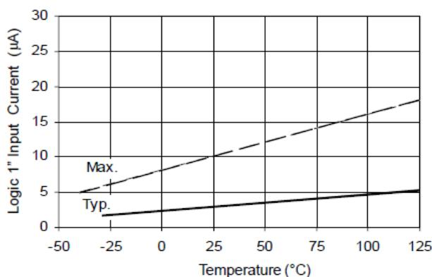
**Figure 19A. Logic "1" Input Current vs. Temperature**
