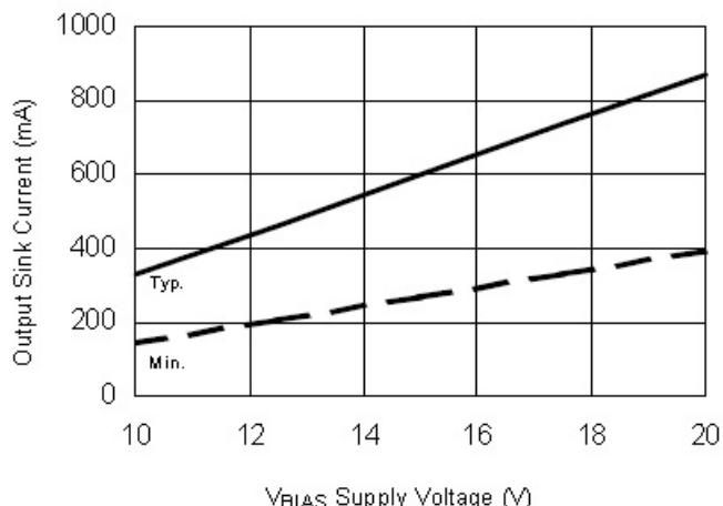
**Figure 24B. Output Sink Current vs. Supply Voltage**
