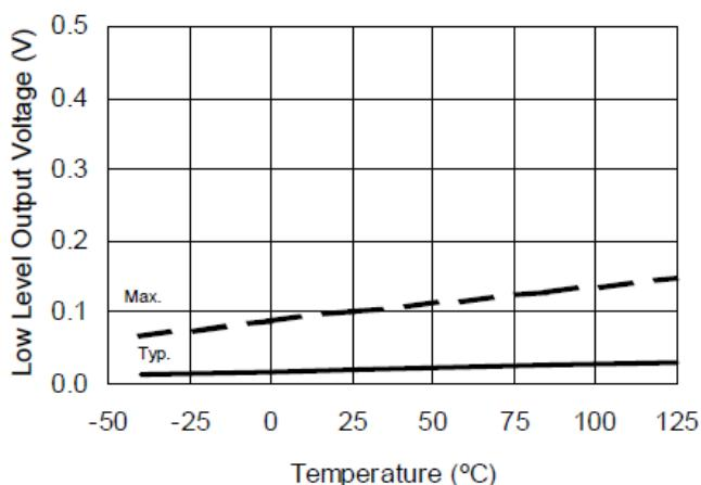
**Figure 15A. Low Level Output Voltage vs. Temperature**
