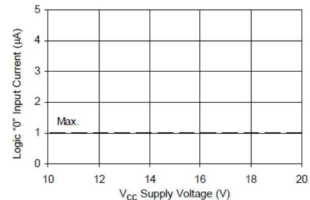
**Figure 20B. Logic "0" Input Current vs. Voltage**
