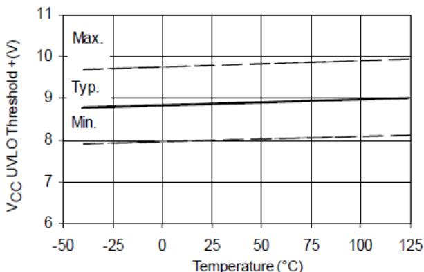
**Figure 21A. V<sub>CC</sub> Undervoltage Threshold(+) vs. Temperature**
