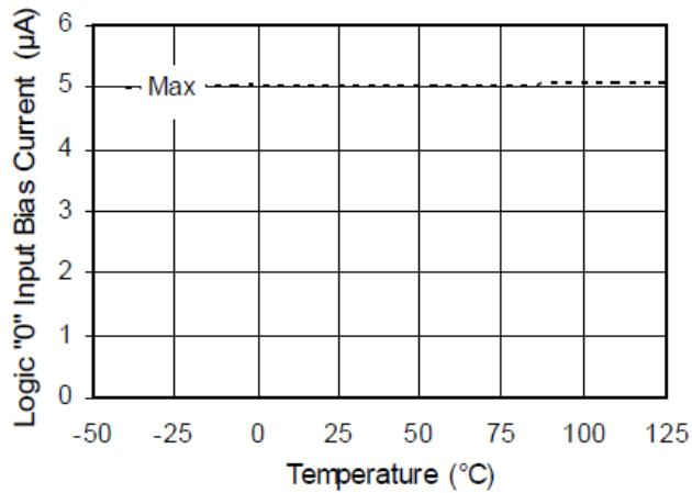
**Figure 13A. Logic "0" Input Bias Current vs. Temperature**
