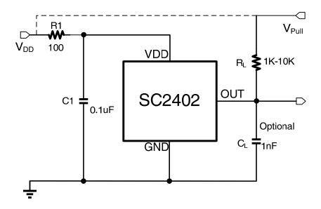
The SC2402 contains an on-chip voltage regulator and can operate over a wide supply voltage range. In applications that operate the device from an unregulated power supply, transient protection must be added externally. For applications using a regulated line, EMI/RFI protection may still be required. R1 is for improved CI performance, and could be 100 or 200  $\Omega$  typically.
