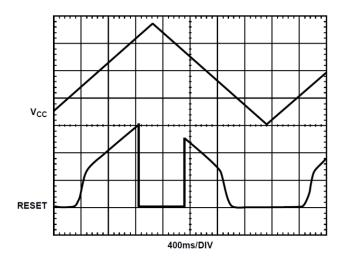
Figure 7. RESET Output Voltage vs. Supply Voltage
