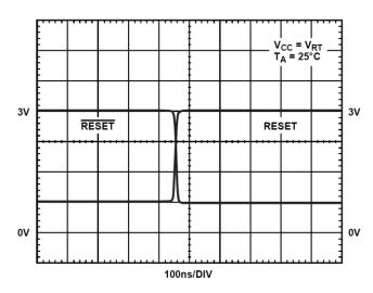
Figure 10. RESET, RESET Assertion
