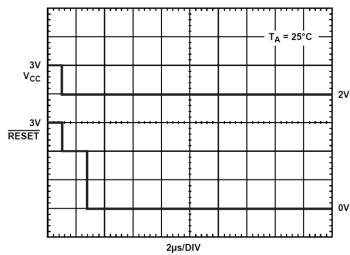
Figure 12. CBM706R/CBM706S/CBM706T and the CBM708R/CBM708S/CBM708T RESET Response Time
