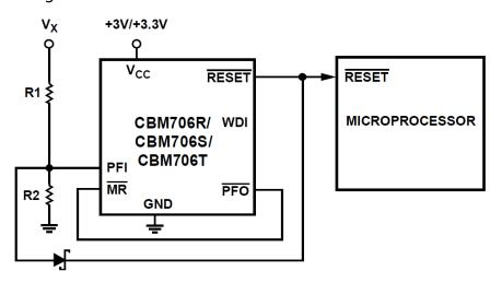
Figure 22. Monitoring 3 V/3.3 V and an Additional Supply,  $V_X$
