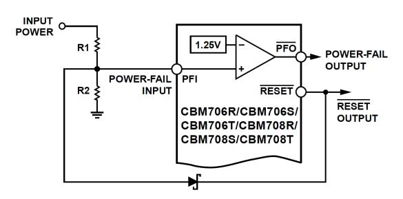
Figure 17. Power Fail Comparator
