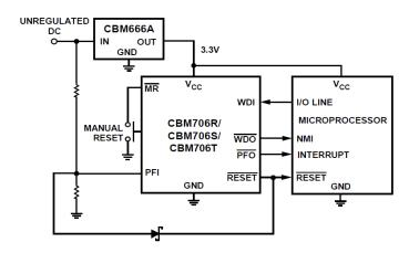
Figure 20. Typical Application Circuit
