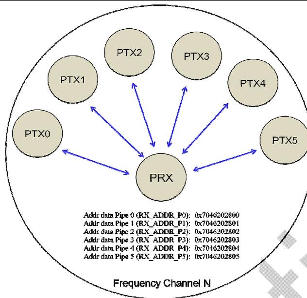
Figure 7.10 Example of data pipe addressing in MultiSlave
