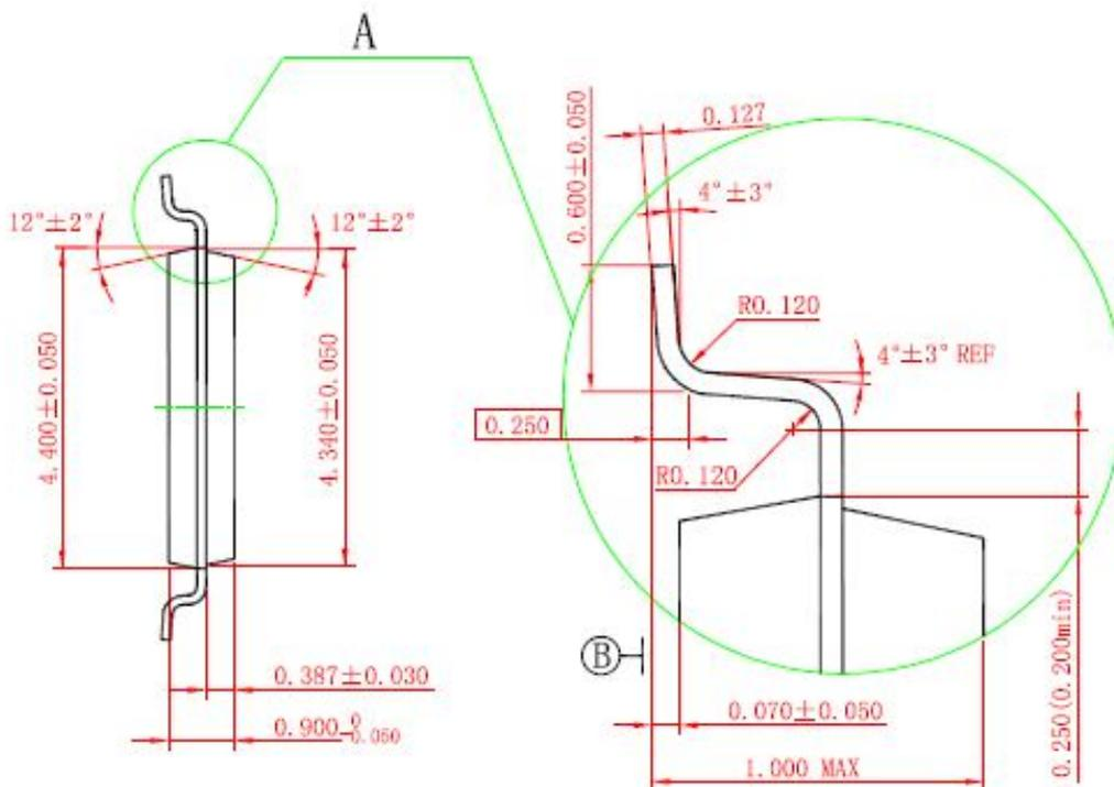
**10.1.3 Uses the Sop16 package, with mAtt tin plating.**
