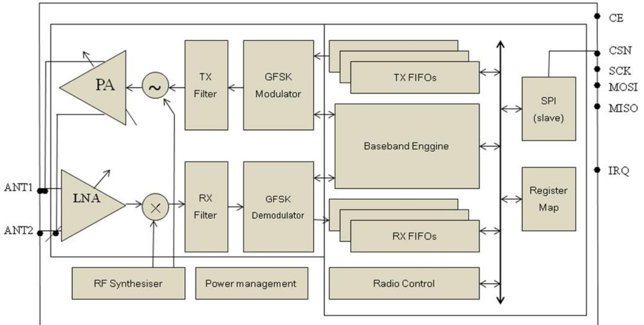
Figure1.1 SE8R01 block diagram
