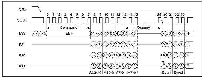
Figure 46 Quad I/O Fast Read Sequence Diagram (SPI, M5-4≠ (1, 0))
