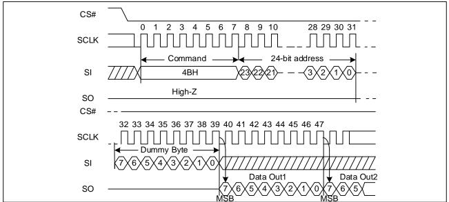
Figure 84 Read Unique ID Sequence Diagram (SPI)
