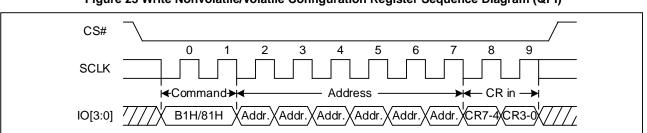
Figure 25 Write Nonvolatile/Volatile Configuration Register Sequence Diagram (QPI)
