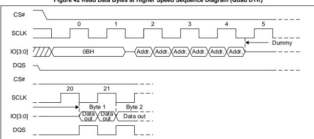
Figure 42 Read Data Bytes at Higher Speed Sequence Diagram (Quad DTR)
