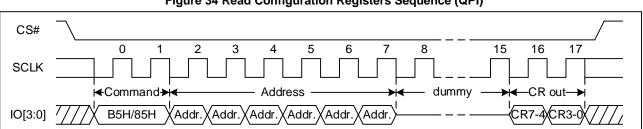
Figure 34 Read Configuration Registers Sequence (QPI)
