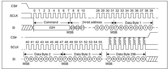
Figure 55 Page Program Sequence Diagram (SPI)
