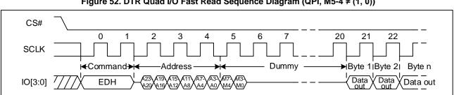
Figure 52. DTR Quad I/O Fast Read Sequence Diagram (QPI, M5-4 ≠ (1, 0))
