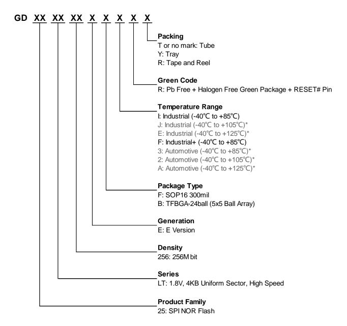
\*This datasheet applies to temperature range I: Industrial (-40°C to +85°C) and F: Industrial+ (-40°C to +85°C) only. Please contact GigaDevice sales for extended temperature industrial products and automotive products.
