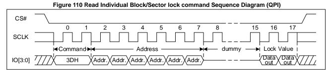
Note: The device default is in 24-bit address mode. For 4-Byte mode, the address length becomes 32-bit.
