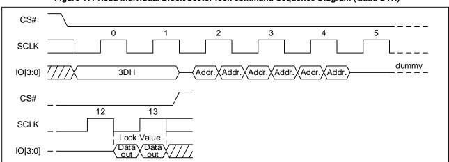
Figure 111 Read Individual Block/Sector lock command Sequence Diagram (Quad DTR)
