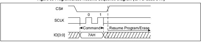
Figure 93 Program/Erase Resume Sequence Diagram (QPI & Quad DTR)
