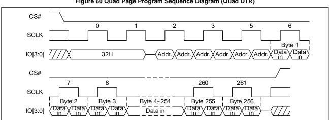
Figure 60 Quad Page Program Sequence Diagram (Quad DTR)
