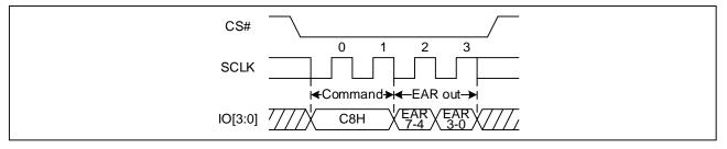
Figure 38 Read Status Register or flag register Sequence Diagram (Quad DTR)
