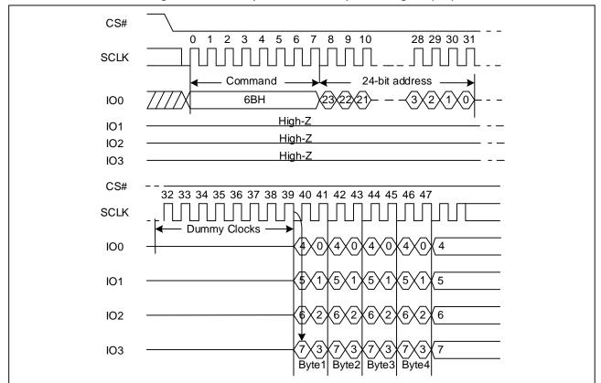
Figure 43 Quad Output Fast Read Sequence Diagram (SPI)
