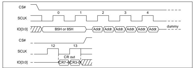
Note: The device default is in 24-bit address mode. For 4-Byte mode, the address length becomes 32-bit.
