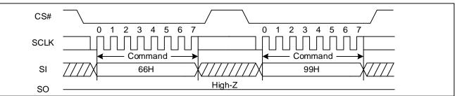
Figure 116 Enable Reset and Reset command Sequence Diagram (SPI)
