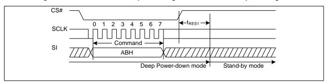
Figure 25. Release Power-Down/Read Device ID Sequence Diagram
