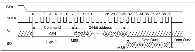
Figure 7. Read Data Bytes Sequence Diagram
