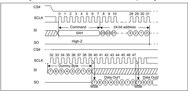
Figure 37. Read Serial Flash Discoverable Parameter command Sequence Diagram
