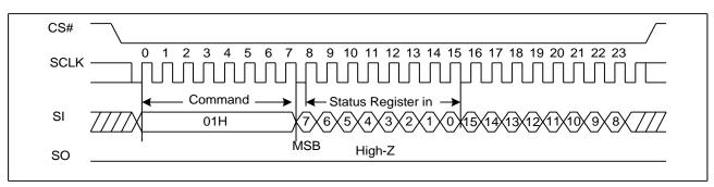
Figure 5. Write Status Register Sequence Diagram
