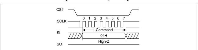
Figure 3. Write Disable Sequence Diagram
