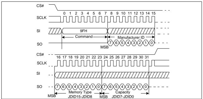
Figure 27. Read Identification ID Sequence Diagram
