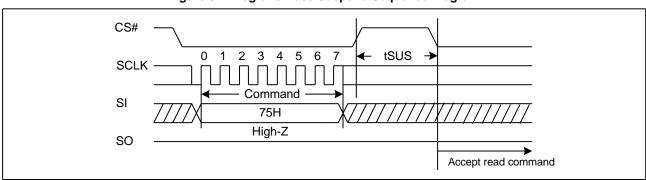
Figure 31. Program/Erase Suspend Sequence Diagram
