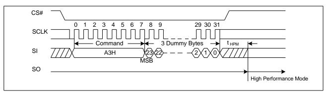
Figure 28. High Performance Mode Sequence Diagram
