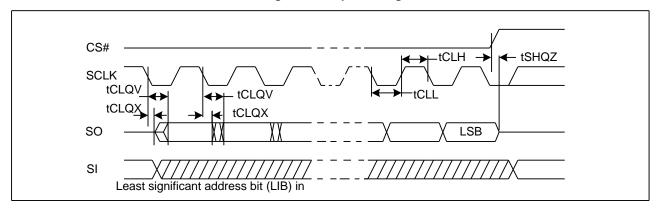
Figure 42. Resume to Suspend Timing Diagram
