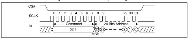
Figure 20. 32KB Block Erase Sequence Diagram
