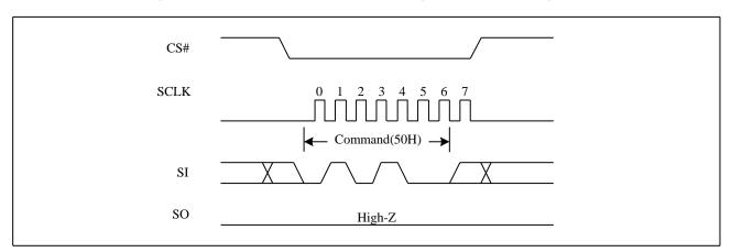
Figure 6. Write Enable for Volatile Status Register Sequence Diagram
