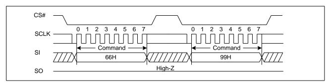
Figure 36. Enable Reset and Reset command Sequence Diagram
