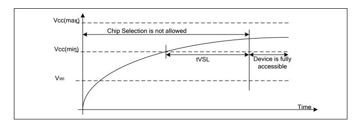
Table6. Power-Up Timing and Write Inhibit Threshold
