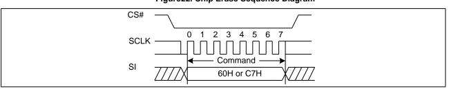
Figure 22. Chip Erase Sequence Diagram
