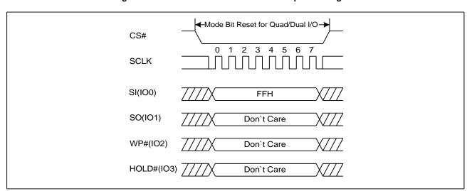
Figure 29. Continuous Read Mode Reset Sequence Diagram
