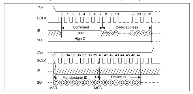
Figure 26. Read Manufacture ID/ Device ID Sequence Diagram
