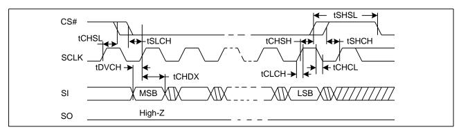
Figure 41. Output Timing
