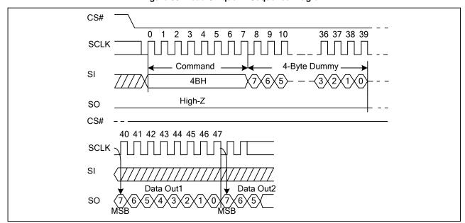
Figure 30. Read Unique ID Sequence Diagram
