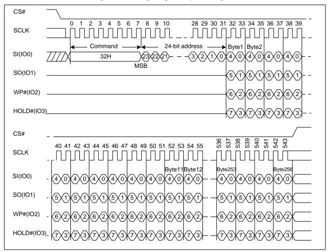
Figure 18. Quad Page Program Sequence Diagram
