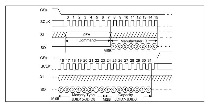
Figure 17. Read Identification ID Sequence Diagram
