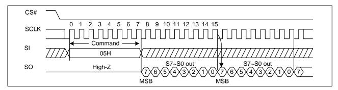
Figure 3. Read Status Register Sequence Diagram
