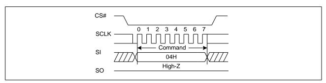
Figure 2. Write Disable Sequence Diagram
