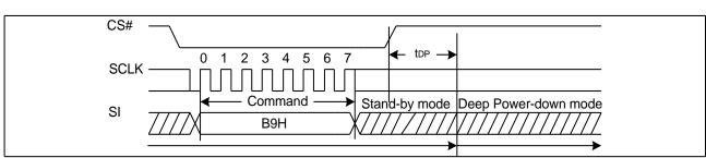
Figure13. Deep Power-Down Sequence Diagram
