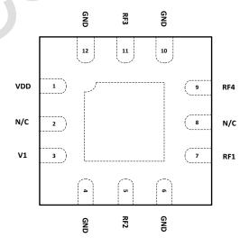
Figure 2. Pin Diagram
