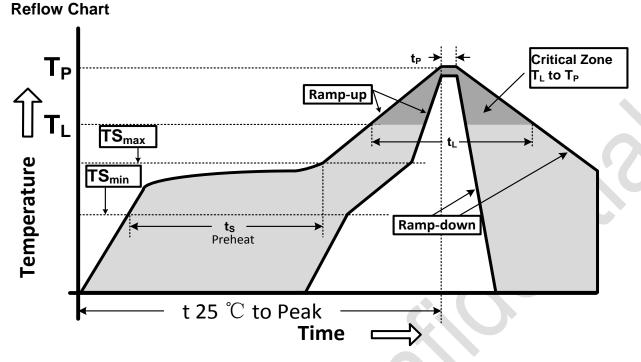
Figure 5. Recommended Lead-Free Reflow Profile
