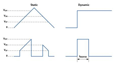
Figure 11.1 Operating principle of the power-on-reset
