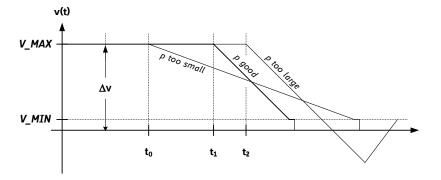
Figure 6.3 Proportionality parameter *p* and outline of velocity profile(s)
