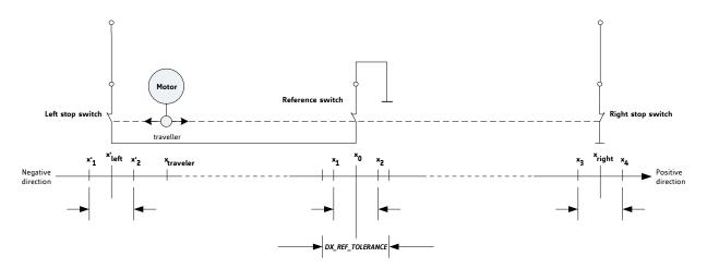
Figure 7.1 Triple switch configuration left stop switch - reference switch - right stop switch
