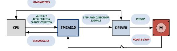
SYSTEM WITH TMC4210 AND TMC2660
