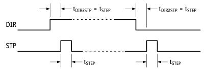
Figure 8.1 Step/Dir timing (en\_sd = 1; step\_half = 0)
