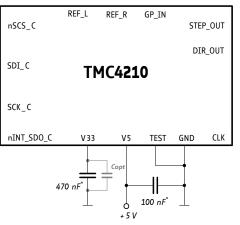
\* Capacitors should be placed as close as possible to the chip.
