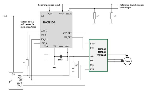
Figure 4.1 TMC4210 application environment with TMC260, TMC261 or TMC2660.
