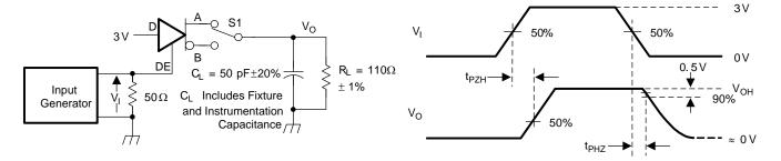
D at 3 V to test non-inverting output, D at 0 V to test inverting output.
