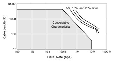
Figure 21. Cable Length vs Data Rate Characteristic
