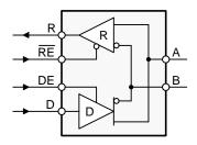
a) Independent driver and receiver enable signals
