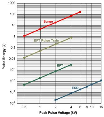
Figure 25. Comparison of Transient Energies
