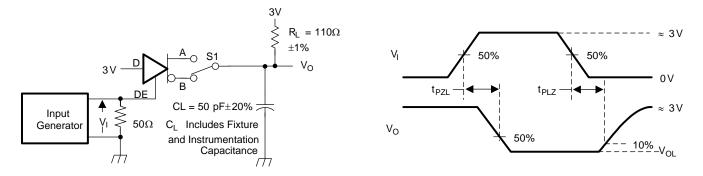
D at 0 V to test non-inverting output, D at 3 V to test inverting output.
