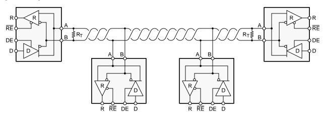
Figure 20. Typical RS-485 Network With 65HVD7x Transceivers
