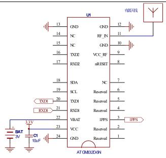
2.7.2 Passive antenna solutions (In RF\_IN input of the module increased one level of LNA)
