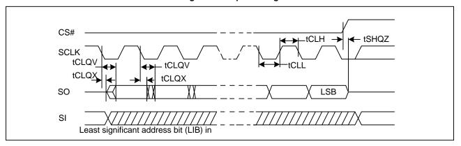
Figure 45. Resume to Suspend Timing
