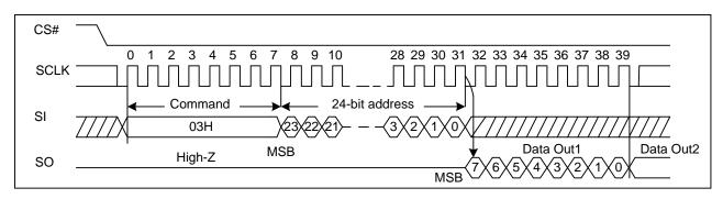
Figure 7. Read Data Bytes Sequence Diagram
