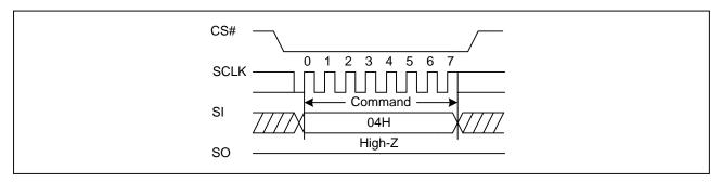
Figure3a. Write Disable Sequence Diagram (QPI)
