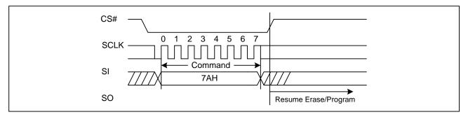
Figure 29a. Program/Erase Resume Sequence Diagram (QPI)
