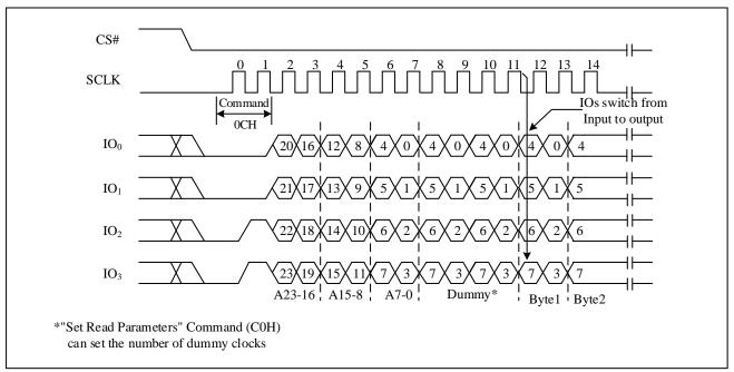
Figure 35. Burst Read with Wrap command Sequence Diagram
