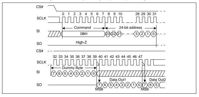
Figure 8. Read Data Bytes at Higher Speed Sequence Diagram
