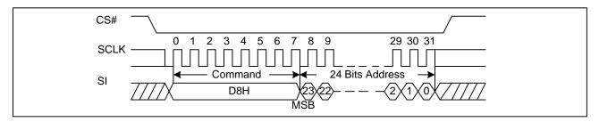
Figure19a. 64KB Block Erase Sequence Diagram (QPI)
