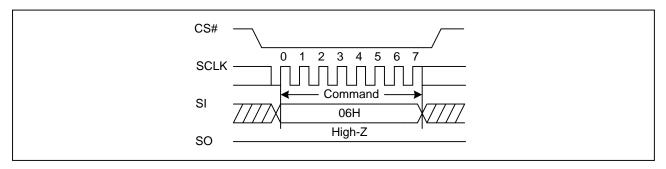
Figure2a. Write Enable Sequence Diagram (QPI)
