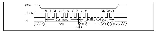
Figure 18a. 32KB Block Erase Sequence Diagram (QPI)
