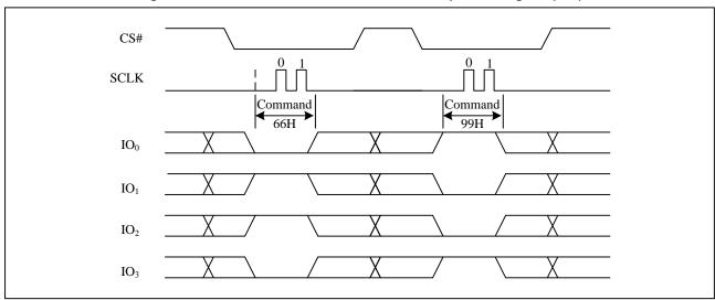
Figure 38a. Enable Reset and Reset command Sequence Diagram (QPI)
