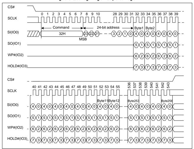
Figure16.Quad Page Program Sequence Diagram
