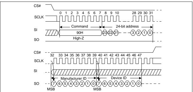
Figure 24. Read Manufacture ID/ Device ID Sequence Diagram
