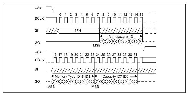
Figure 27. Read Identification ID Sequence Diagram
