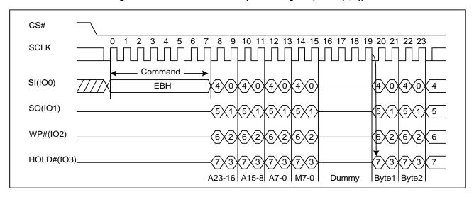
Figure 12. Quad I/O Fast Read Sequence Diagram (M5-4≠ (1, 0))
