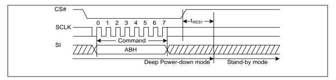
Figure22a. Release Power-Down Sequence Diagram (QPI)
