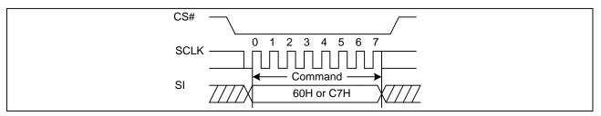
Figure 20a. Chip Erase Sequence Diagram (QPI)
