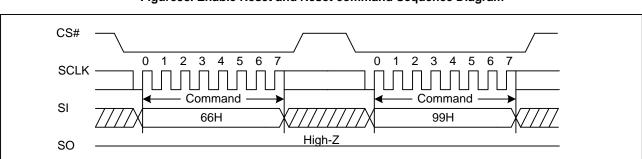
Figure 38. Enable Reset and Reset command Sequence Diagram
