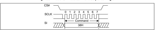
Figure 36. Enable QPI mode command Sequence Diagram
