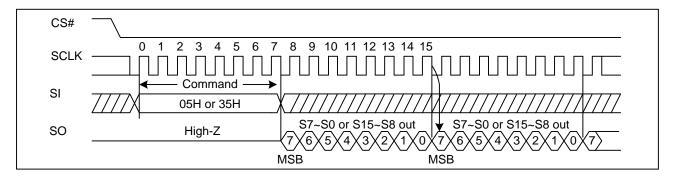
Figure5a. Read Status Register Sequence Diagram (QPI)
