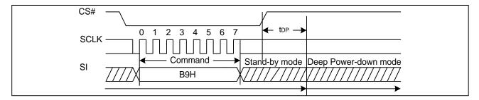
Figure21a. Deep Power-Down Sequence Diagram (QPI)
