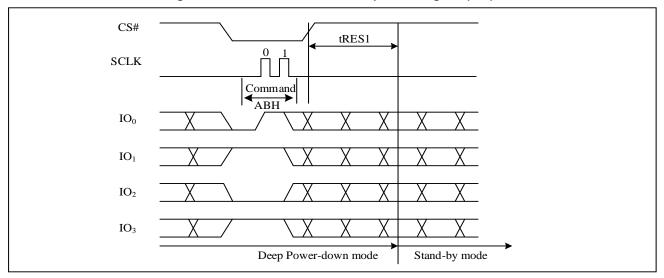
Figure 23. Release Power-Down/Read Device ID Sequence Diagram
