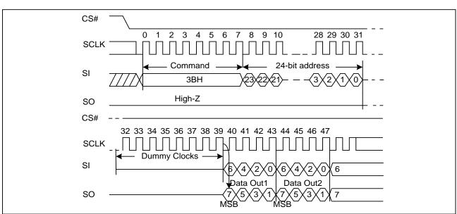
Figure 9. Dual Output Fast Read Sequence Diagram
