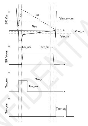
Figure 9.2: SR Control Block Sequencing Diagram
