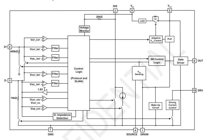
Figure 8.1: iW661 Functional Block Diagram
