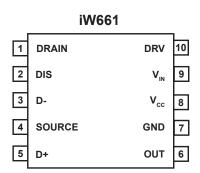
Figure 4.1: 10-Lead MSOP Package
