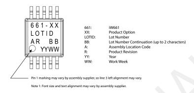
Figure 12.1: Top Marking for the iW661
