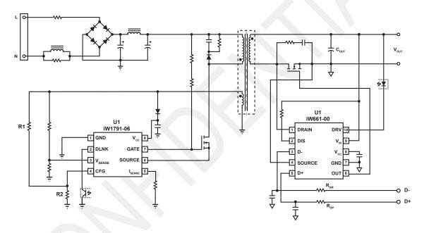
Figure 9.3: iW661 Typical Application Circuit for Multi-Level Output Voltage and Current with RC Filtering at D+/D-. (Using iW1791-06 as Primary-side Controller. Achieving <20mW No-Load Power Consumption).
