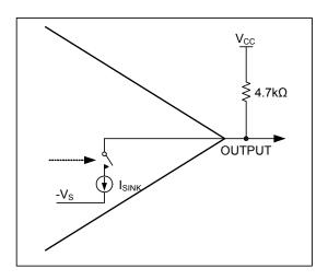
Figure 1. Open Drain Output Stage Circuitry
