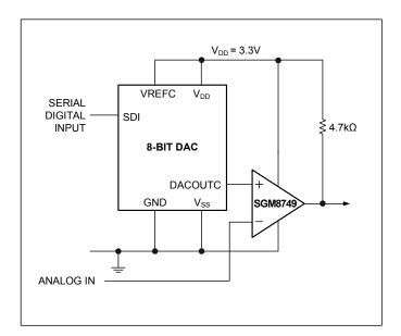
Figure 2. 3.3V Digitally Controlled Threshold Detector
