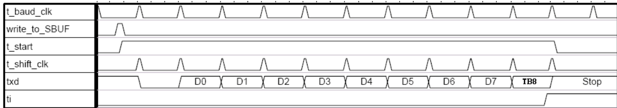
Fig. 8-5: Transfer Mode 2 and Mode 3
