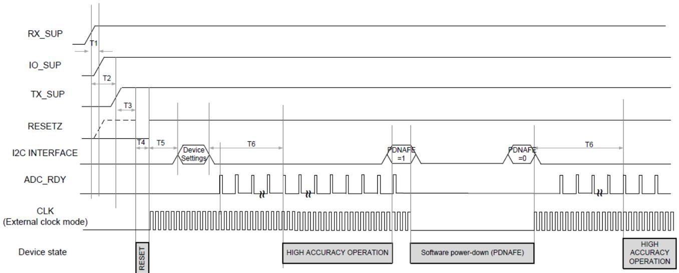
Figure 68. Power Supply Sequencing, Device Initialization, and Software Powerdown Timing
