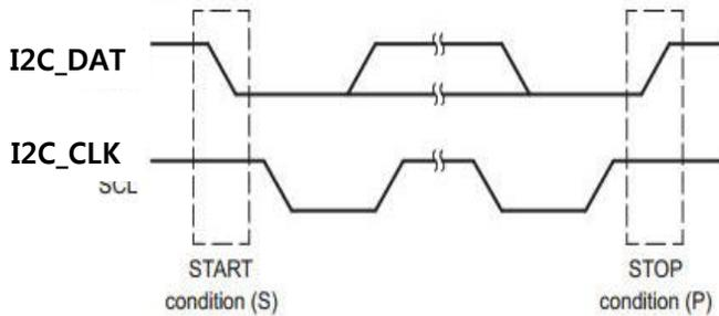
Figure 8. Start and Stop Condition
