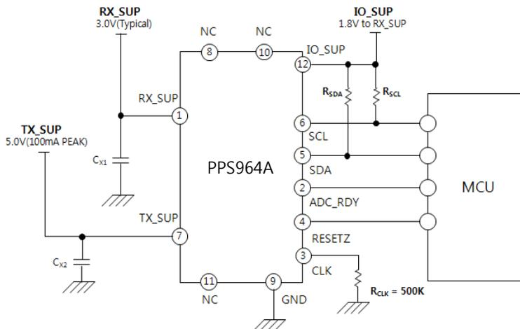
Figure 69. Hardware pin connection diagram in internal oscillator mode
