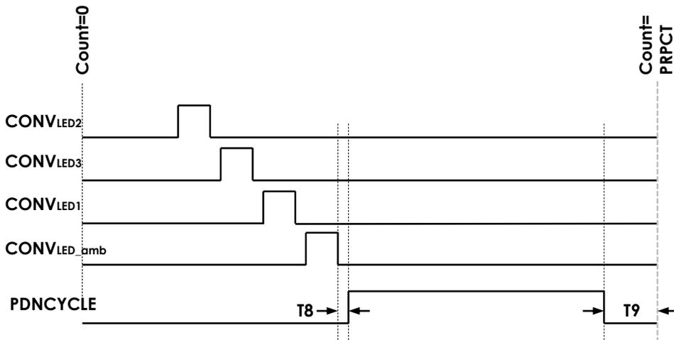
Figure 14. Dynamic Powerdown Timing Diagram
