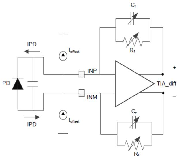
With the photodiode connected as shown, In figure 5, the output code of the PPS964A would be positive with the offset cancellation DAC set to zero ( $I_{offset}=0$ ). With  $I_{offset}$  set negative ( $POL\_OFFDAC=1$ ), a DC offset can be subtracted from the signal, and the AC signal could be amplified with a higher gain than would be otherwise possible.
