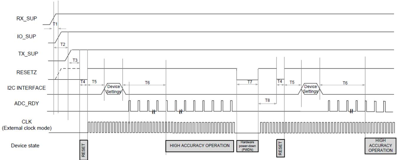
Figure 67. Power Supply Sequencing, Device Initialization, and Hardware Powerdown Timing
