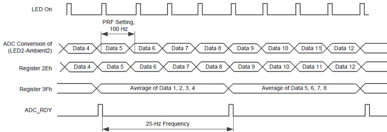
Figure 16. Decimation mode enabled timing diagram (Decimation factor =4, PRF = 100 Hz)
