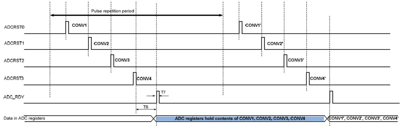
Figure 13. ADC\_RDY Generation Scheme
