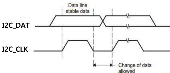
Figure 7. Allowed Window for Data Transition
