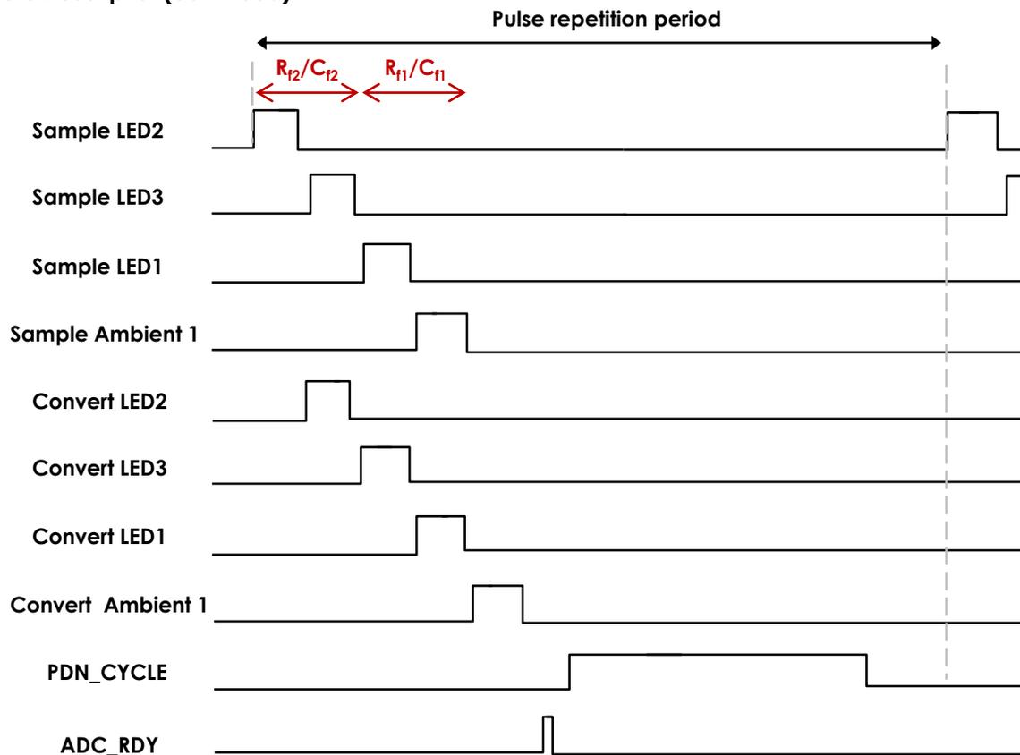
Figure 4. Illustration on Sequence of Four Phases of Sampling and conversion
