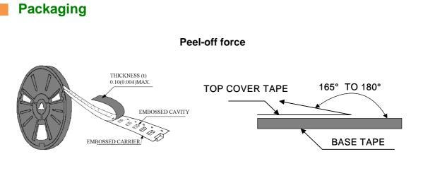
The peel off force of cover tape is 10 to 70 grams in the arrow direction.
