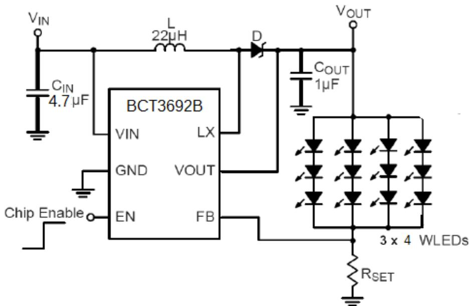
Figure 2. Application for Driving 3 X 4 WLEDs
