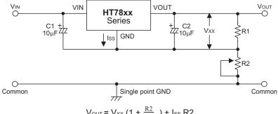
$$V_{OUT} = V_{XX} (1 + \frac{R2}{R1}) + I_{SS} R2$$
