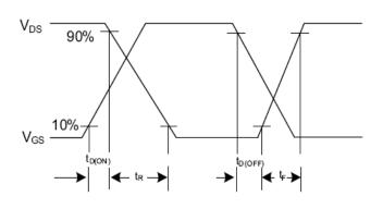
Fig. 2.2 Switching Waveforms
