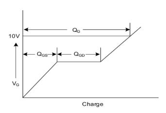
Fig. 3.2 Gate Charge Waveform
