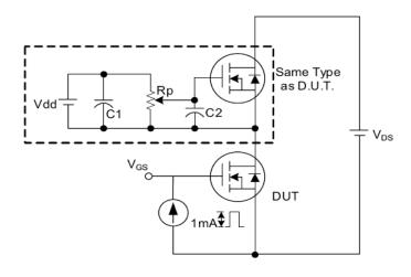
Fig. 3 . 1 Gate Charge Test Circuit
