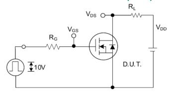
Fig. 2.1 Switching Test Circuit
