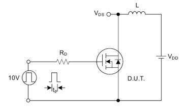
Fig. 4.1 Unclamped Inductive Switching Test Circuit
