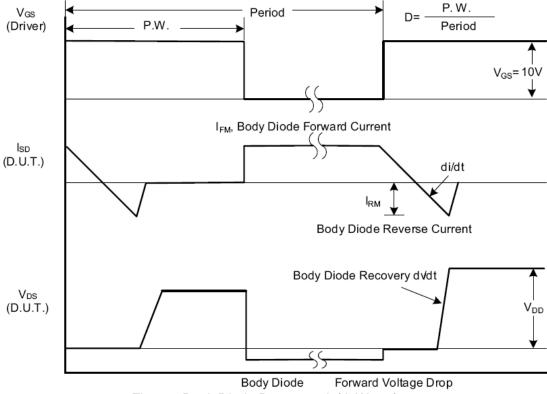
Fig. 1.2 Peak Diode Recovery dv/dt Waveforms
