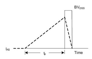
Fig. 4.2 Unclamped Inductive Switching Waveforms
