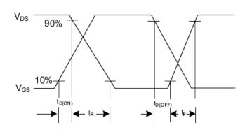
Fig. 2.2 Switching Waveforms
