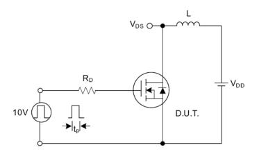
Fig. 4.1 Unclamped Inductive Switching Test Circuit
