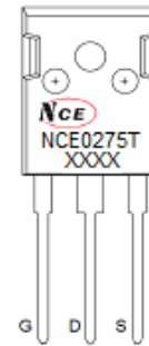
Marking and pin assignment
