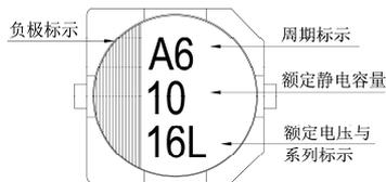
$\phi D = 8 \sim 10 \text{ mm}$
